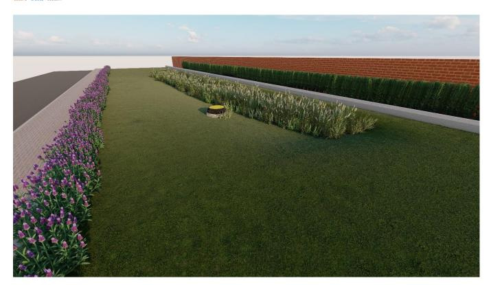
Once paved with the media and top soil, the only visible sign of the swale is the inspection shaft cover, which doubles up as a ventilation shaft and an entry port for excessive storm-water runoff in event of really heavy burst. The whole system has Zero land costs because you can install other MEP services above the blocks.
