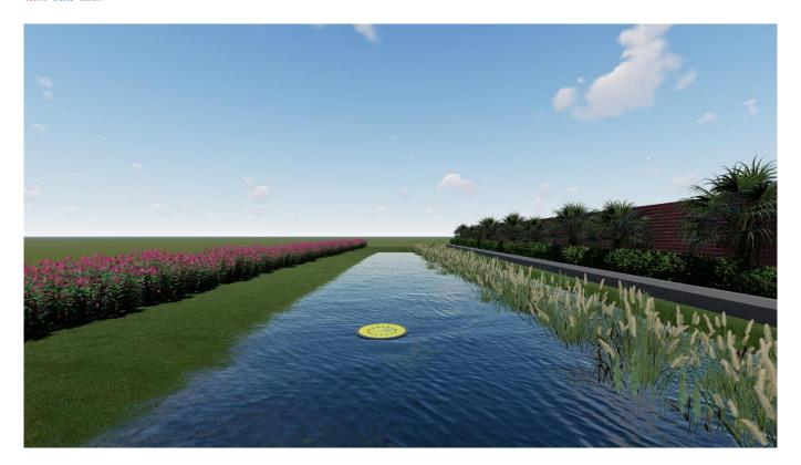
Water starts to get drained directly through the yellow shaft cover, only when the surface collections have reached a particular height in the bioswale.
