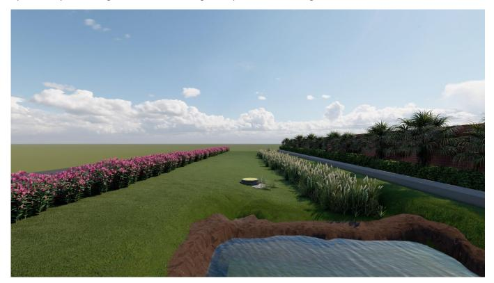
As an essential part of SUDS strategy the underdrained swales meet all the three cardinal principles- Soak the Rain, Spread it fast and Slow down the flow. The Geocellular blocks provide temporary or permanent detention, transportation and where required infiltration into the ground for recharge.
