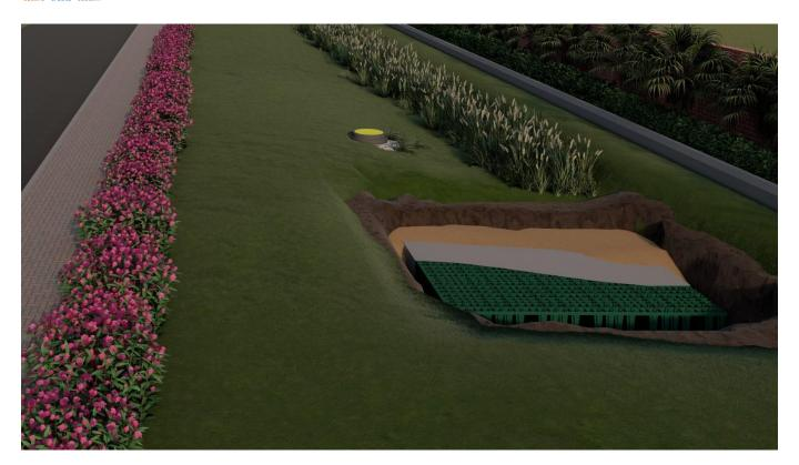
Our solutions can be designed to handle the heavy downpours, which we now see every now and then, by adding Geocellular soak basins under the green landscape, we can quickly trap pure rainwater in the confines of private aquifers for ground water recharge and possible reuse, right there where it falls.
