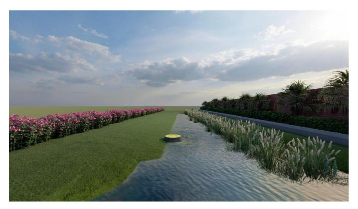
The topography is designed to sweep the rainwater into the plantation beds holding perennials with a good fibrous root system. These beds have transit slopes draining towards shallow ponds at intermittent lengths.
